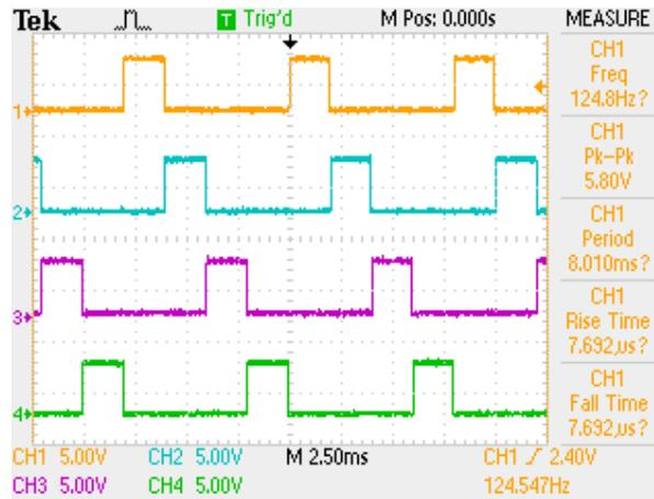
*PICmicro provides anode drive pulses shifted in time for each tube
