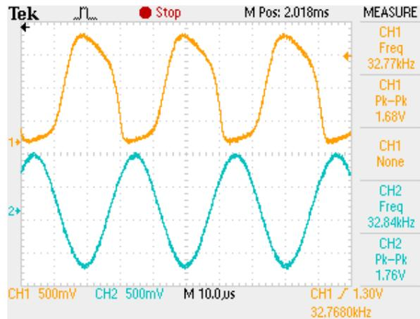
Y1 oscillator waveforms
