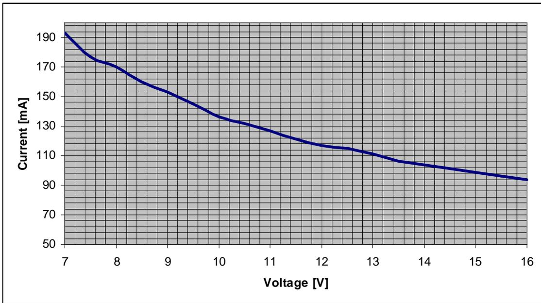
Graph below shows current consumption according to power supply voltage. Tubes' voltage set to 170V. Backlight enabled at full intensity.
