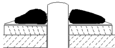
A bad connection is where the solder has not "stuck" to the component lead.
