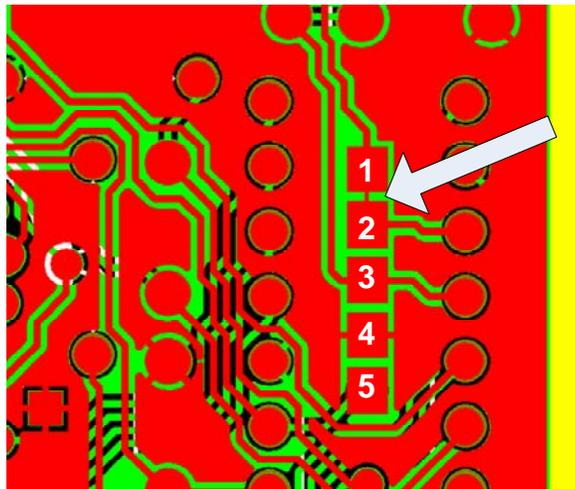
Programming connector has etched jumper between pin #1 and pin #2
