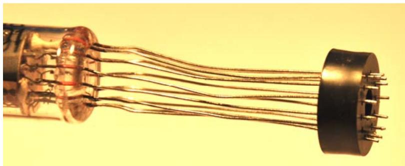
*Placing spacer near the end of wires*
