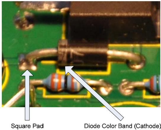
*UF4007 diode placing*
