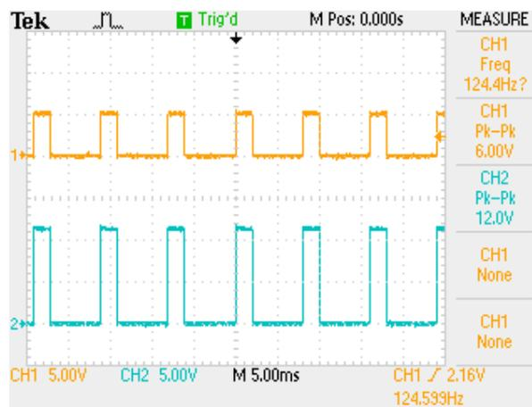
Backlight PWM waveform
