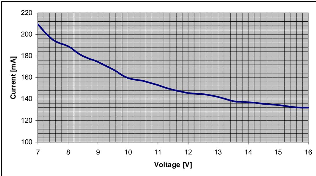
Below is shown power consumption graph according to power supply voltage. Tubes' voltage is set to 170V. Blue line shows power consumption with backlight enabled at full intensity, green without backlight.
