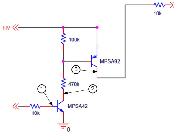
NOTE (x) Waveforms on these points are provided. Number means oscpe channel.
