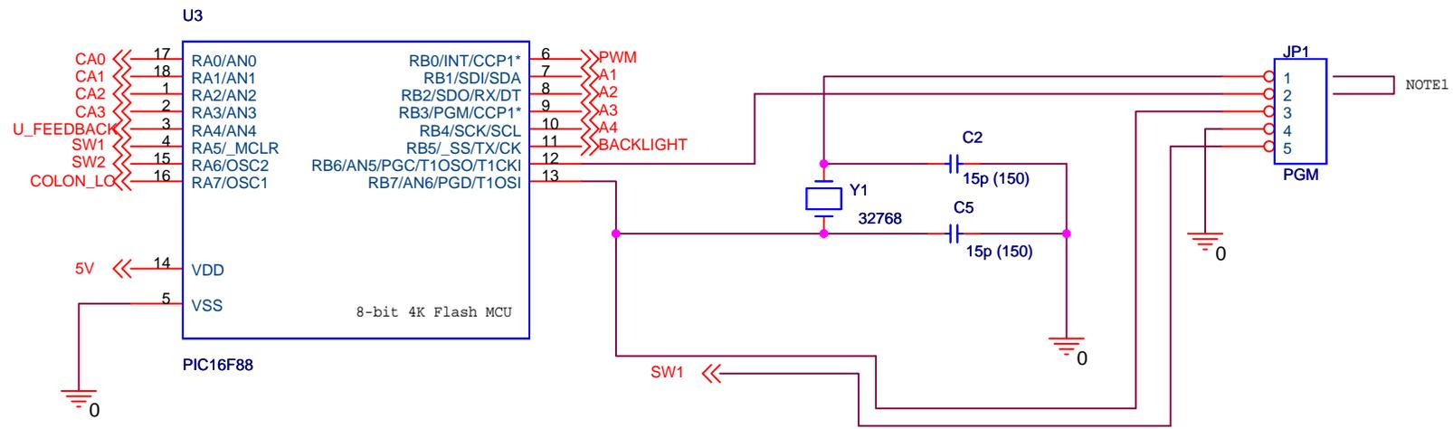
NOTE1 - Jumper between JP1 pin #1 and pin #2 is etched on the PCB. It must be removed during programming otherwise should be left inserted. For more information refer to the user's guide.
