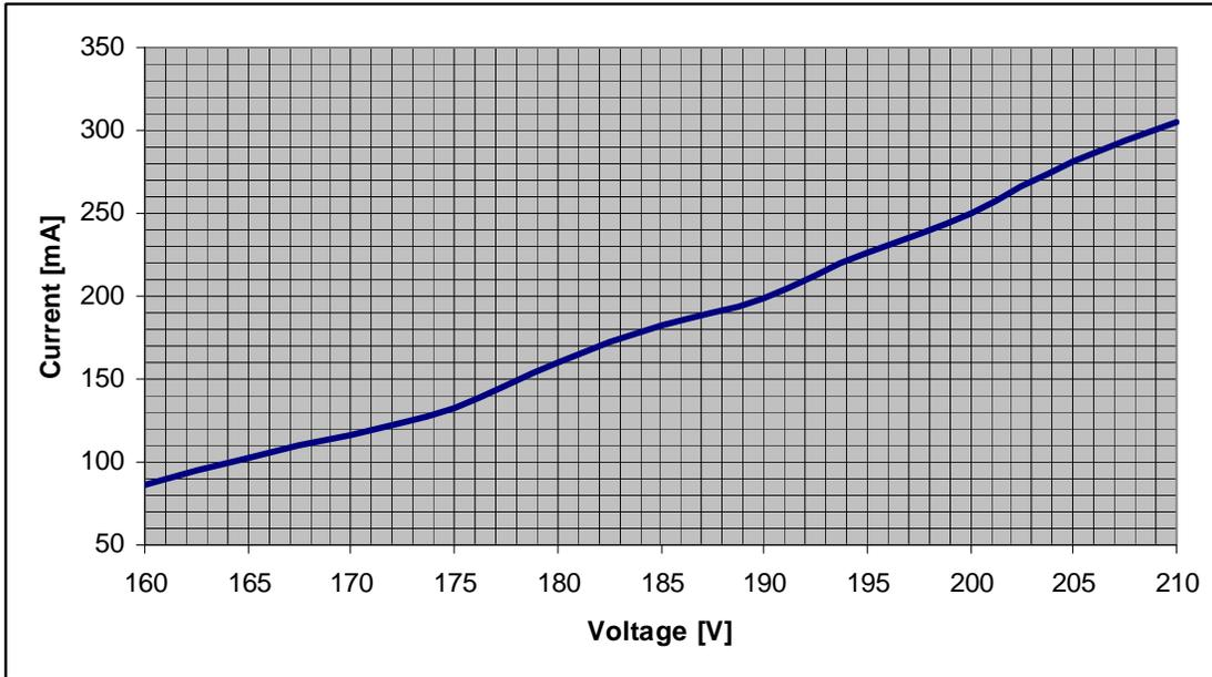
Graph above shows current consumption according tubes' voltage. Power supply set to 12V. Backlight off. Backlight, if enabled at full intensity, adds 24mA to whole range. Please note, voltages above 200V are limited by firmware in order to protect IRF640 MOSFET.
