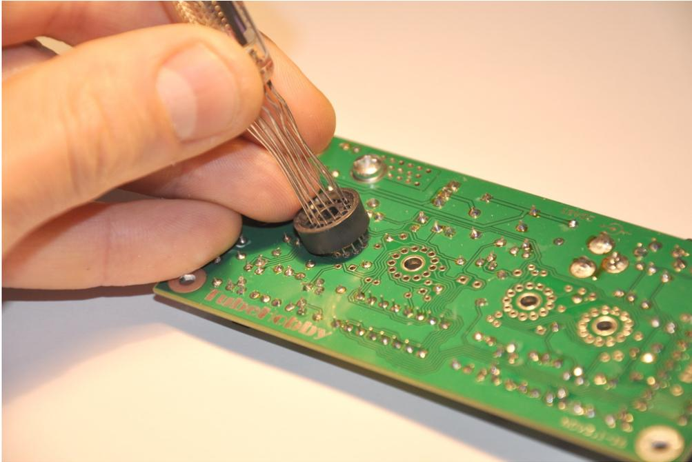
*Insert nixie tube at the angle holding spacer near the end of wires*
