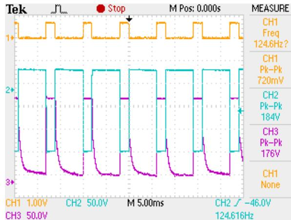
*Anode driver waveforms
