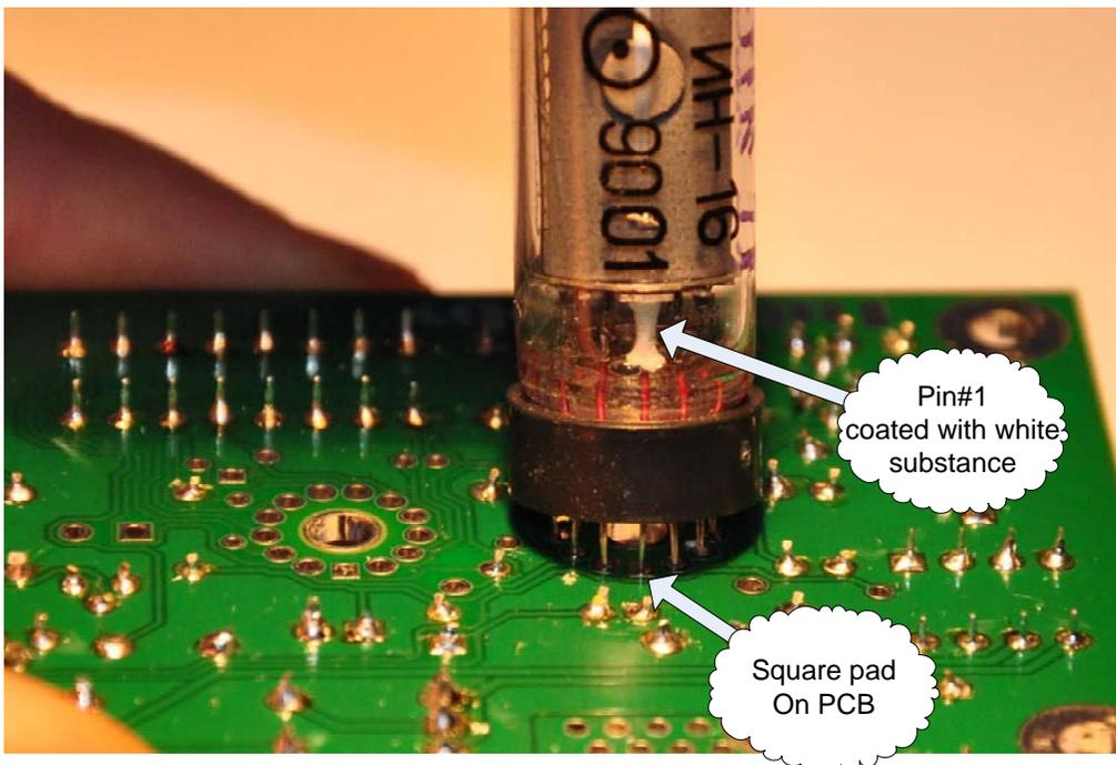
*Pin #1 and footprint verification before soldering*
