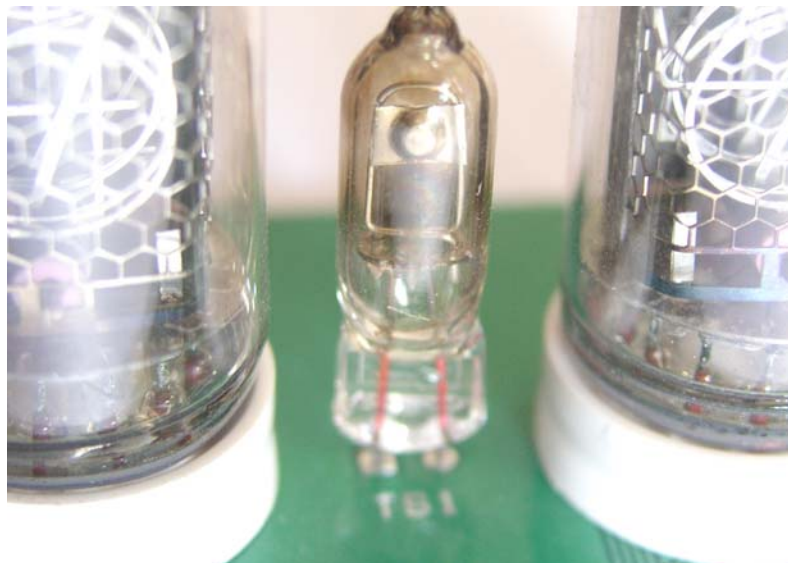
Fig. 7. IN-3 type column separator bulb
